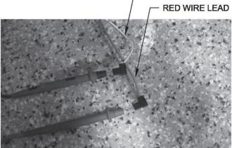
output. A reading under 400 millivolts indicates a bad thermopile, replace the pilot assembly per service procedure ED-II on page 10.
